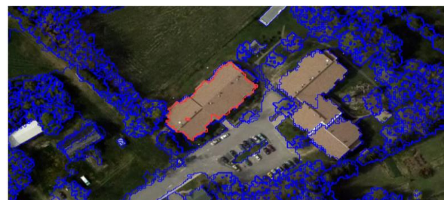
Figure 1: Shows the Object-Based Image Analysis (OBIA) segmentation process[16].
