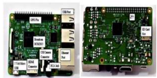
Figure 10: Parts of the Raspberry Pi 3 Model B+
