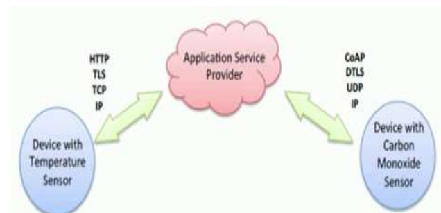
Figure 4: Device to Cloud Communication
