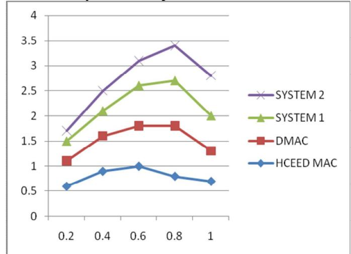
As shown in figure 2 as the arrival rate increases throughput increases more in HCEEDMAC when compared to DMAC, system I, system II . Because of Adaptive power control technique the power is efficiently utilized and more number of users are accommodated in HCEEDMAC protocol when compared with DMAC protocol, system I, system II
