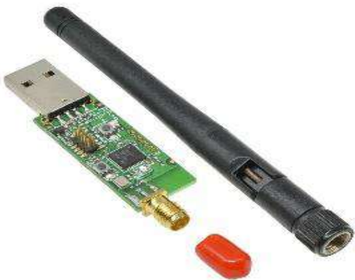
Figure 3: USB RF Transceiver with External Antenna
