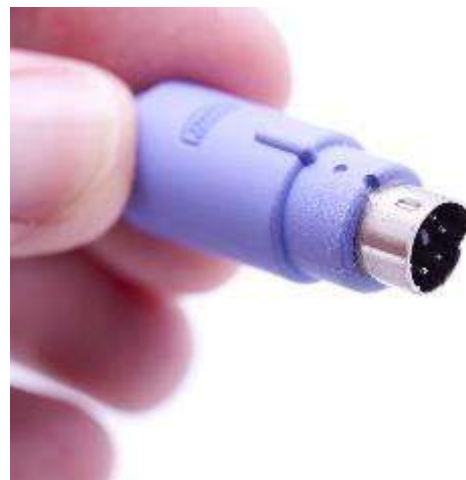
Figure 1: Legacy PS/2 Keyboard Connector
