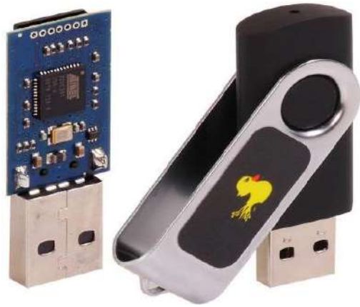
Figure 2: USB Hardware Keylogger Devices
