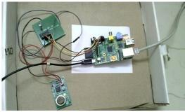
Fig. 5: Sensors connected to GPIO
