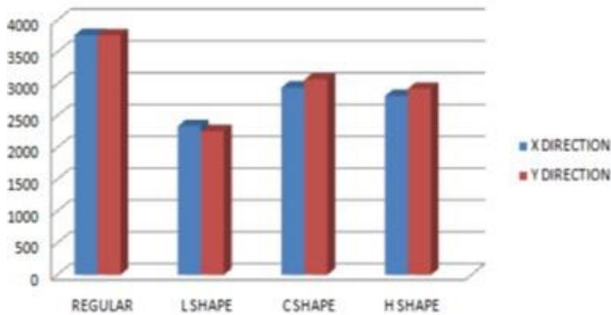
Figure 10: Base shear (Kn) of G+15 storey concrete encased I section column building
