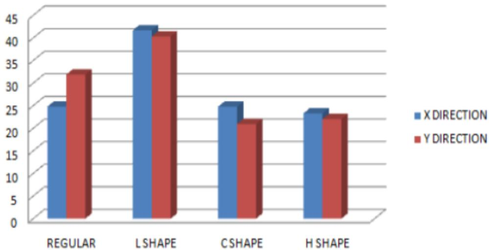
Figure 18: Storey displacement (mm) of G+15 storey conventional column building
