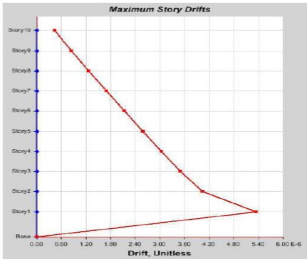
Figure 11: Storey drift of G+10 storey conventional column building
