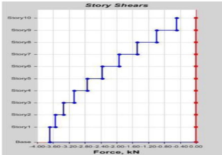
Figure 7: Base shear (kn) of G+10storey conventional column building
