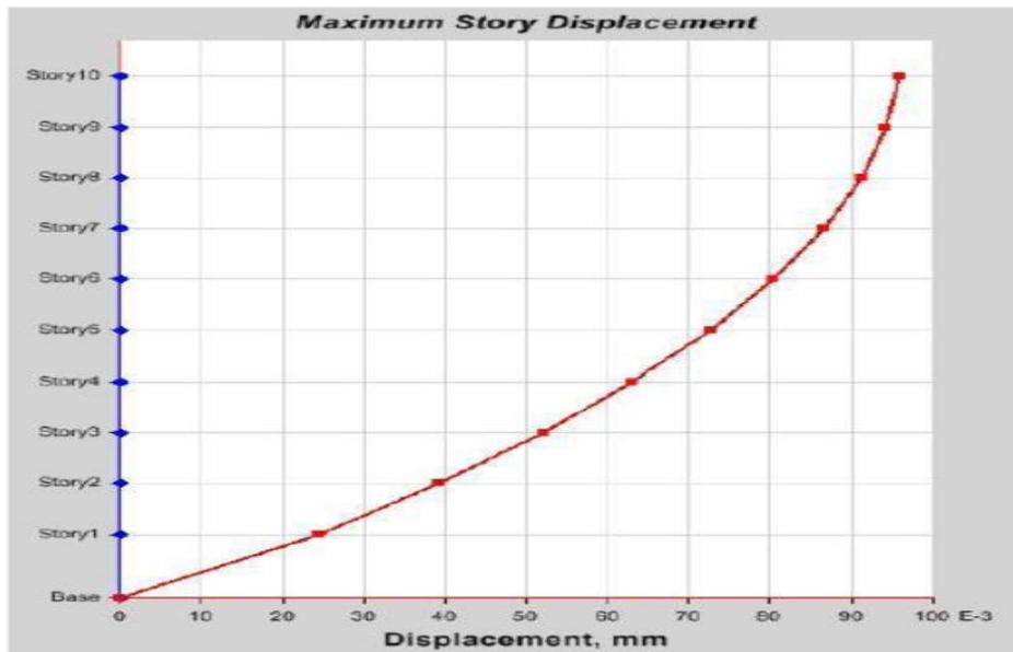
Figure 17: Storey displacement(mm) of G+10 storey concrete encased I section column building
