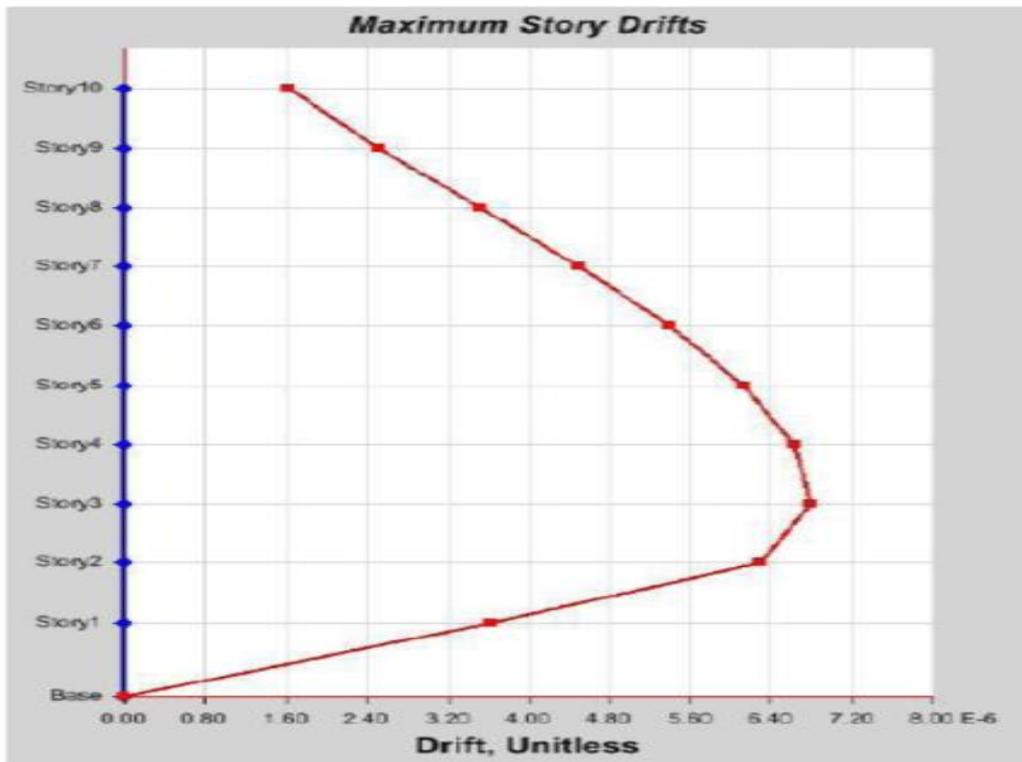
Figure 12: Storey drift of G+10 storey concrete encased I section column building
