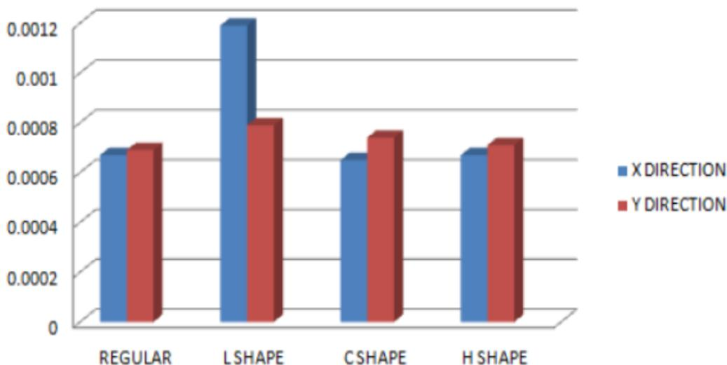
Figure 14: Storey drift of G+15 storey concrete encased I section column building
