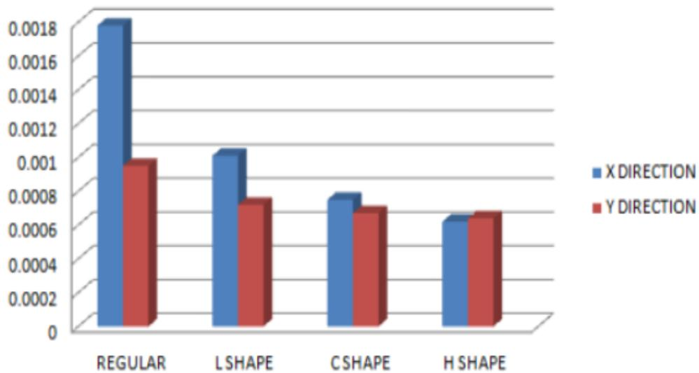
Figure 13: Storey drift of G+15 storey conventional column building
