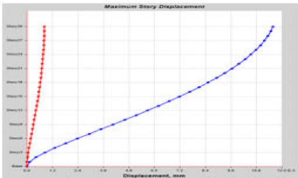
Figure 21: Storey displacement(mm) of G+30 storey concrete encased I section column building
