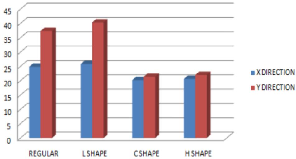
Figure 19: Storey displacement(mm) of G+15 storey concrete encased I section column building
