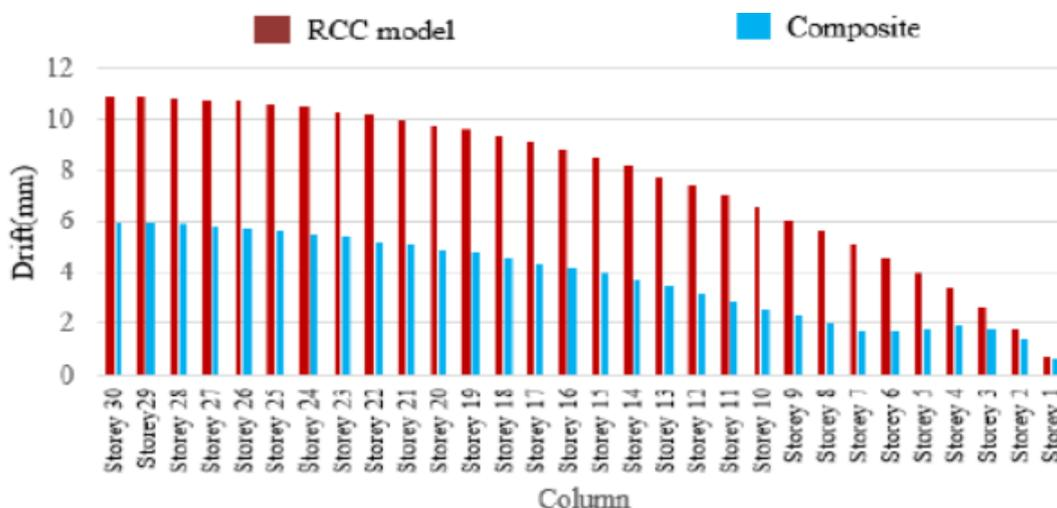
Figure 15: Storey drift of G+30 storey
