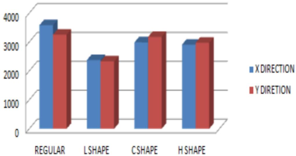
Figure 9: Base shear (kn) of G+15 storey conventional column building
