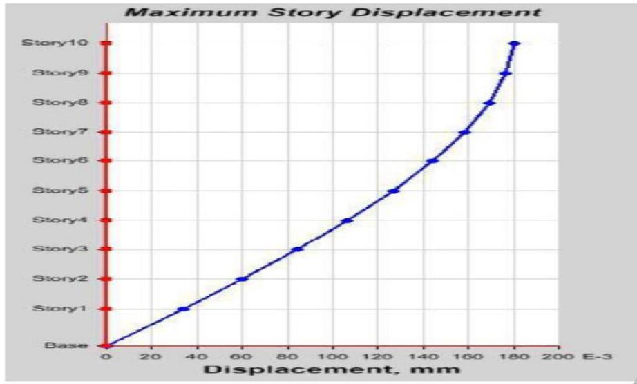
Figure 16: Storey displacement (mm) of G+10storey conventional column building
