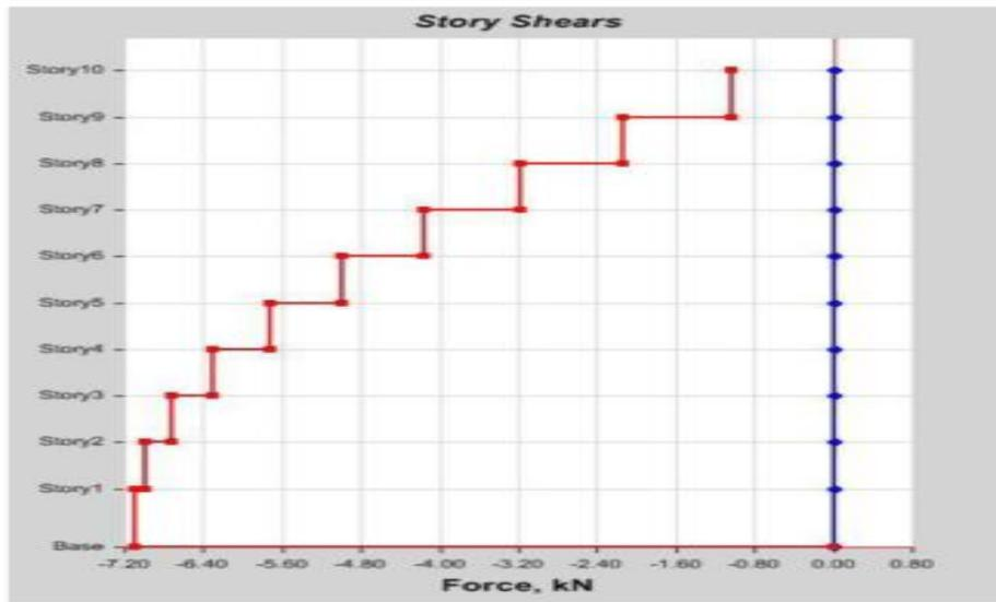
Figure 8: Base shear (Kn) of G+10 storey concrete encased I section column building
