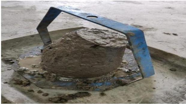
Figure 5: Slump Cone Test
