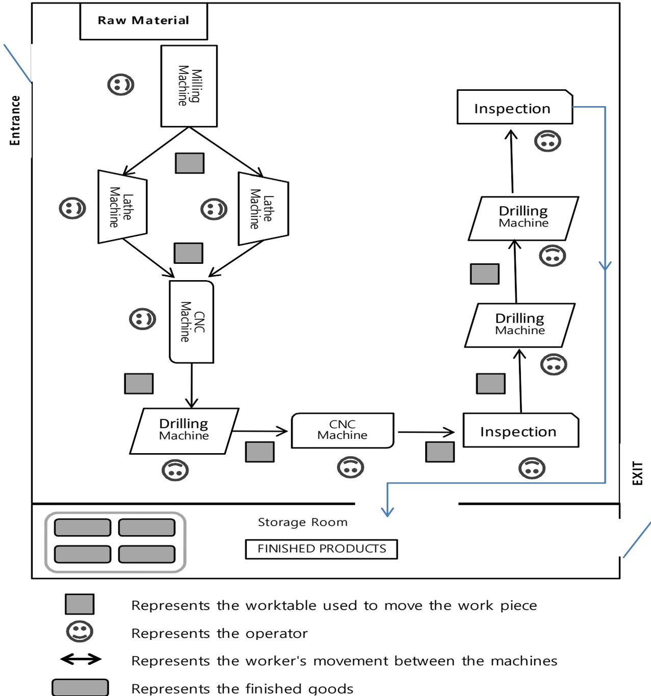
Fig. 4: The process layout prior to improvements
