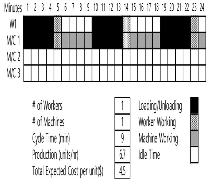
Fig. 2: Prior to changes in phase (4) or (8)
