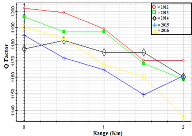
Fig 2: Quality factor of the received signal versus range (different years)
