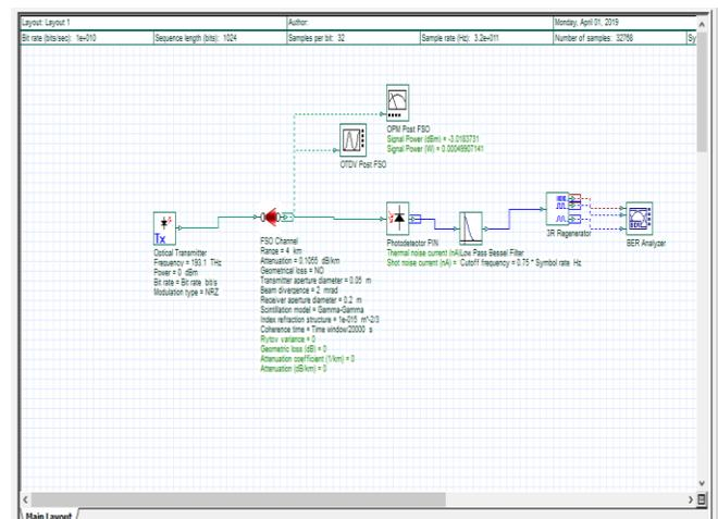
Fig 1: System model analyzing the effect of rain attenuation
