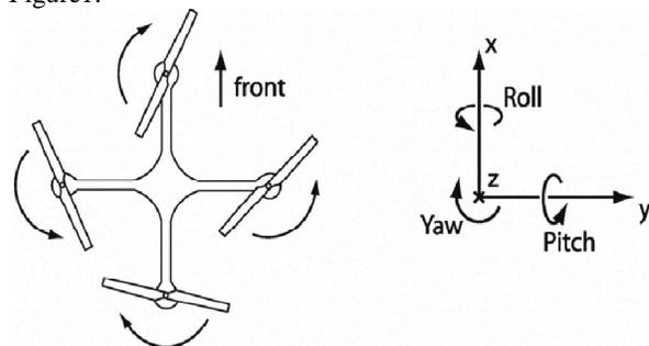
Figure 2: Basic design of the quad copter
