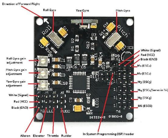
**Figure 3: Stabilization Board**
