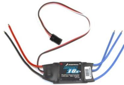
**Figure 4: Electronic Speed Controller (ESC)**
