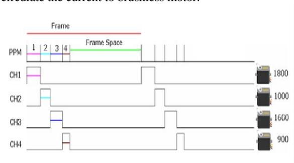
Figure 13: PPM signal send by R.C transmitter
