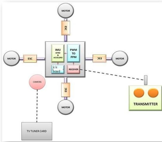
Figure 12: Block diagram of Quad copter
