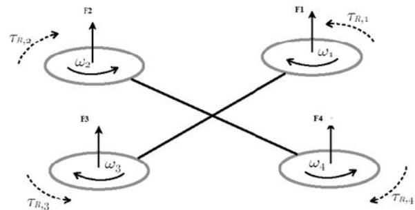
Figure 1: The rotation of propellers
