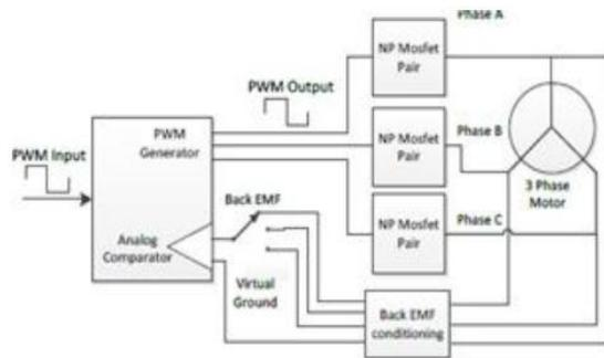
**Figure 5: Internal schematic of ESC**
