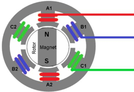
**Figure 6: Internal Structure of Brushless DC Motor**
