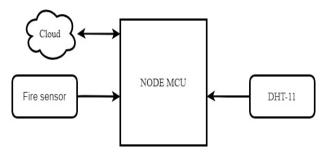
Figure 1: Block diagram of a Fire detection system
