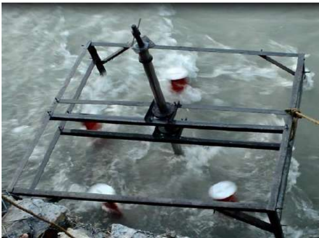
Figure 11: Testing of VAWT in shallow water channel
