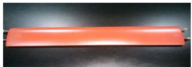
Figure 8: Rotor Blades of Vertical Axis Water Turbine after Fabrication
