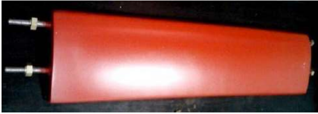
Figure 9: Bolts Inserted in Blades
