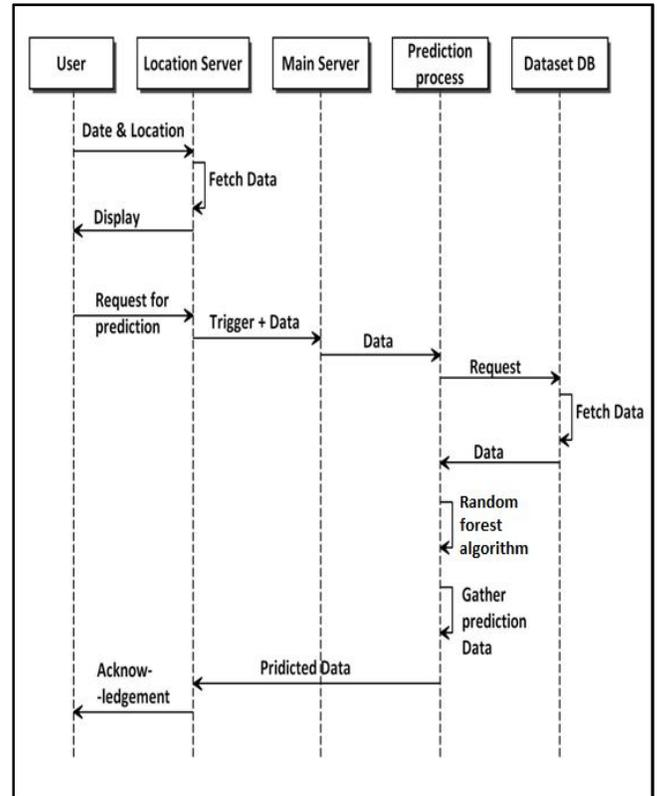
Fig 2: Data transmission in sequence diagram
