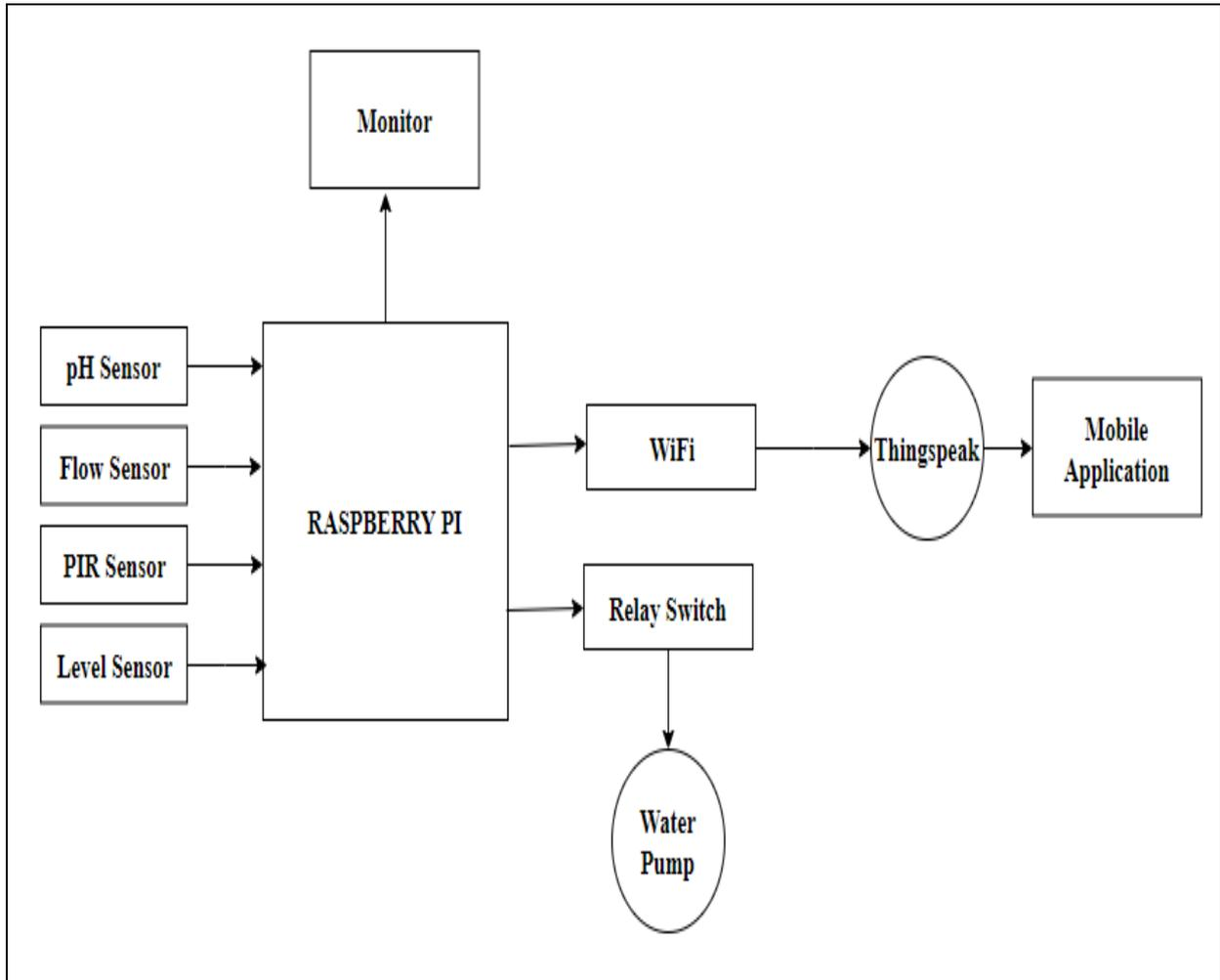
Fig. 1: Block diagram of controller system
