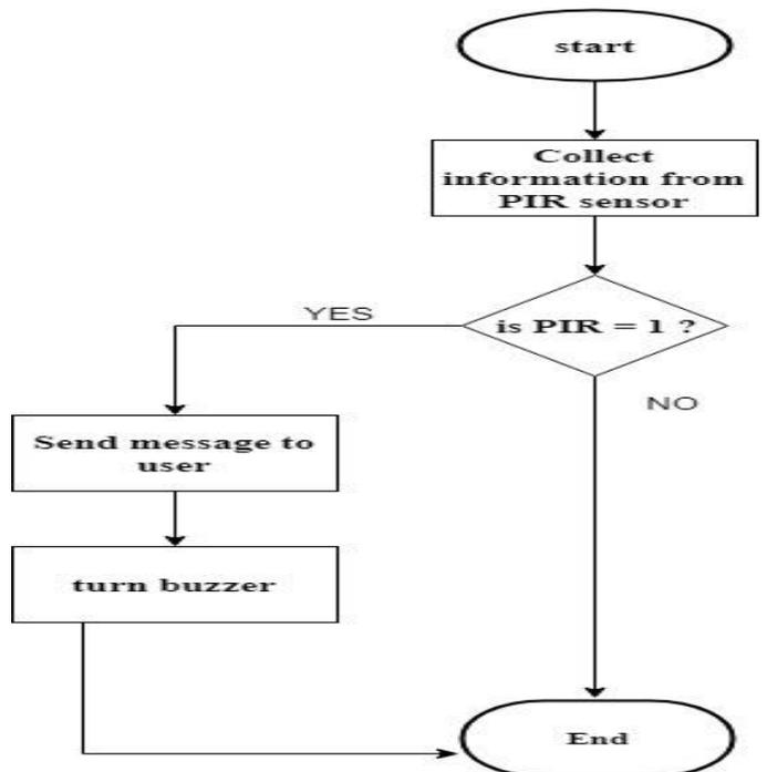
Fig. 6: Control logic for PIR sensor
