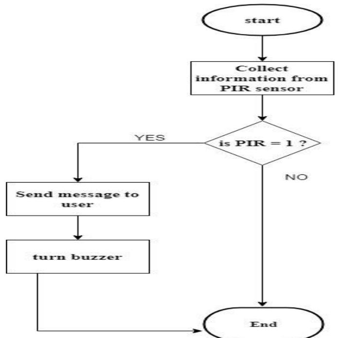
Fig. 6: Control logic for PIR sensor
