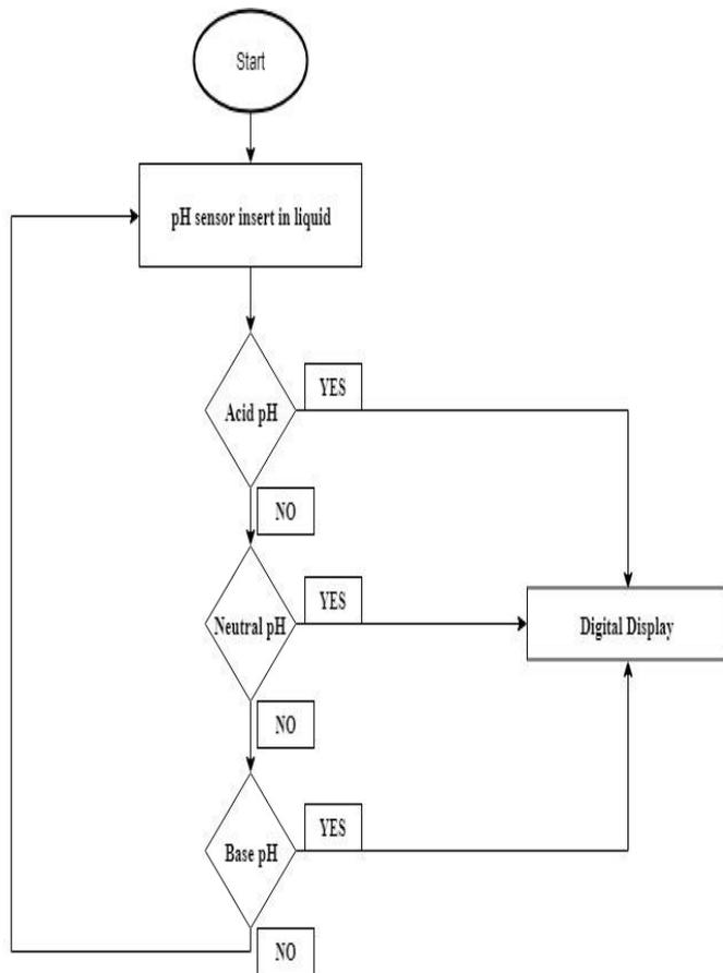
Fig. 5: Control logic for pH sensor
