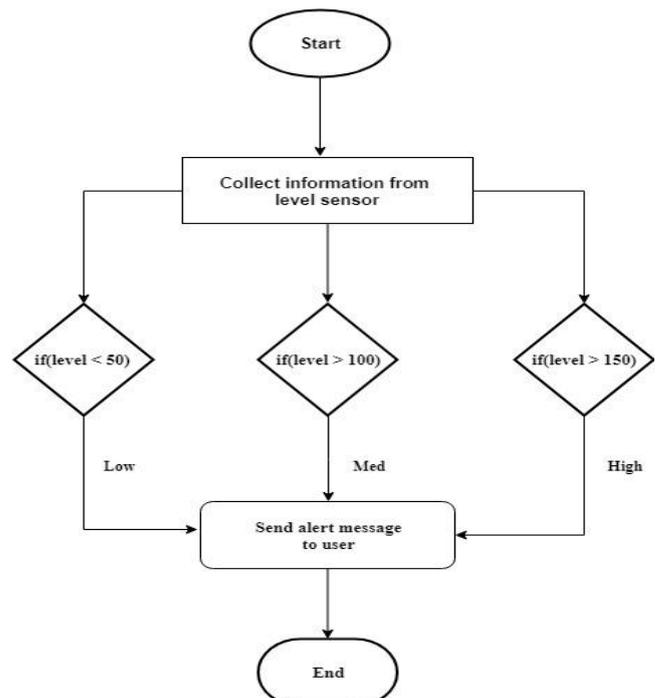
Fig. 2: Control logic for level sensor
