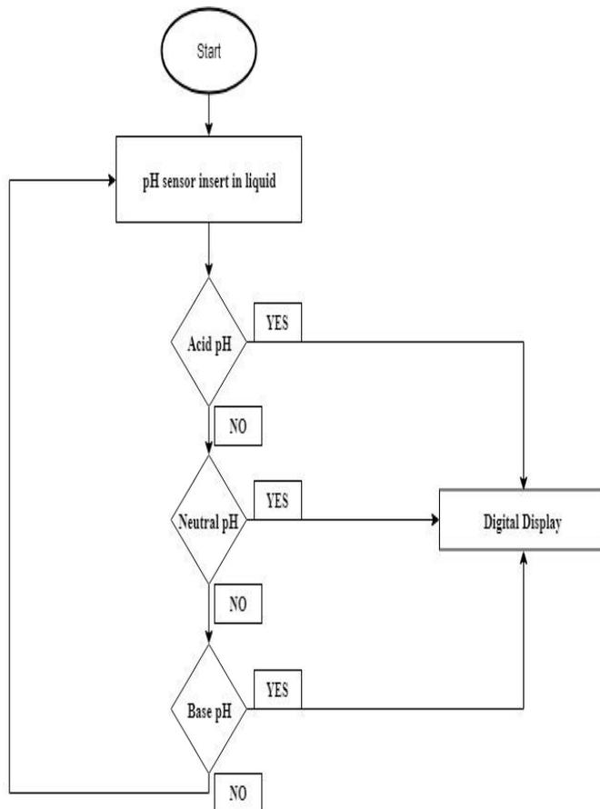
Fig. 5: Control logic for pH sensor
