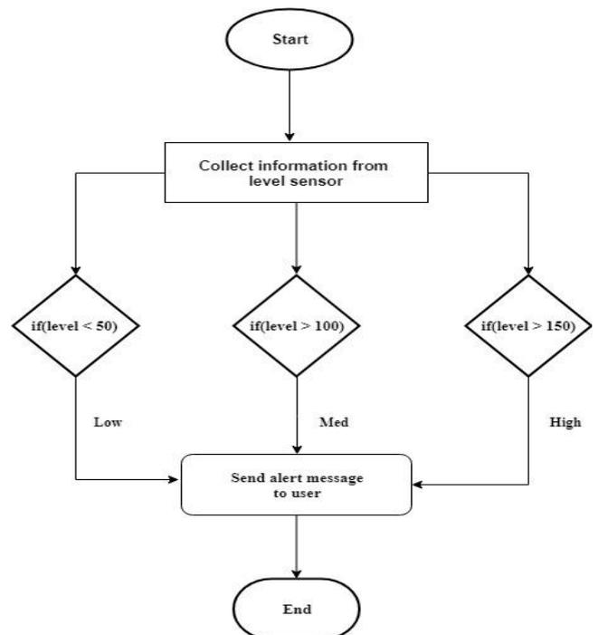
Fig. 2: Control logic for level sensor
