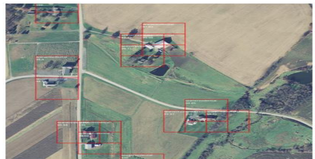
Figure 1: Part of the image from Fig. 3(a) in which the example of object detection is given. In this example, the blocks which have a high probability to contain a sparse residential area are highlighted with red (best view in color)
