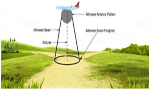
Figure 1: Radio altimeter working principle
