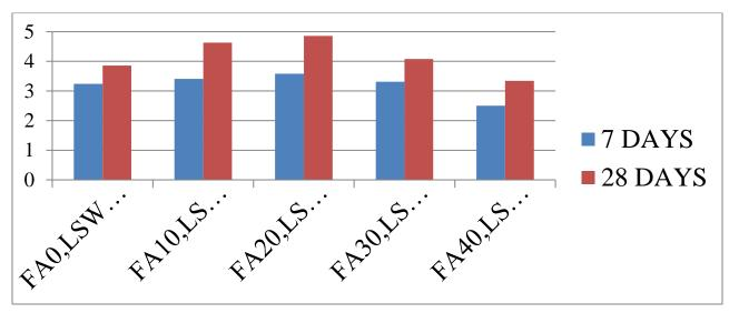
Figure 5: Split tensile test after 7 and 28 days respectively
