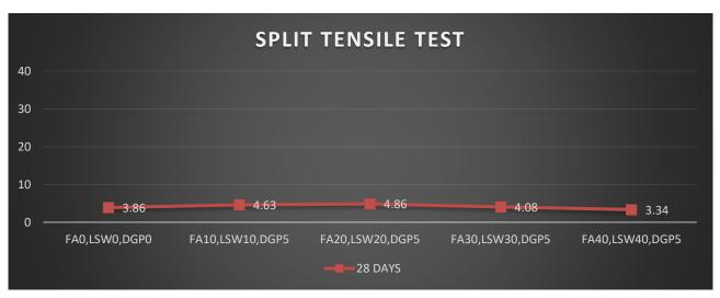
Figure 4: Split tensile test after 28 days
