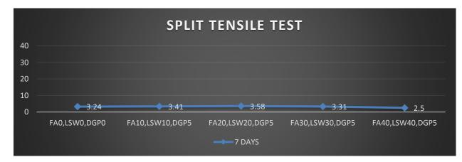
Figure 3: Split tensile test after 7 days
