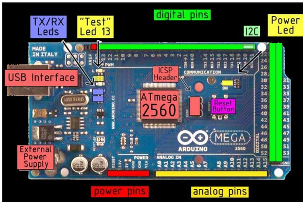
Fig. 3: Arduino mega Board
