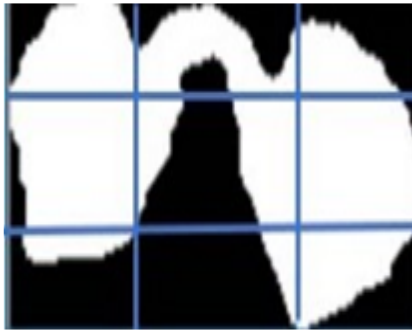
Figure 8: The Hand Pose 'a' in ISL Fragmented by a 3x3 Grid
