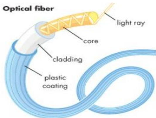
Figure 2 : The Optical Fiber and Their Different Components[6]
