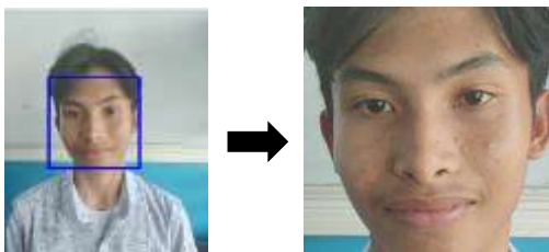
Figure 5: Result of face image detection using the viola-jones algorithm
