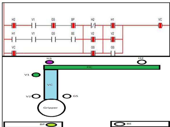
Fig.6: Program Of Vertical Conveyor Circuit
