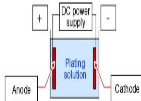
Fig.1: Electroplating of metal [5][11]
