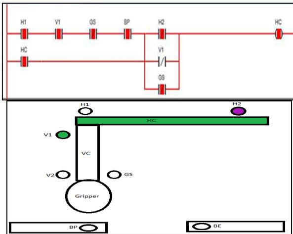
Fig.5: Program of Horizontal Conveyor Circuit
