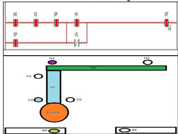
Fig.7 Program Of Gripper circuit
