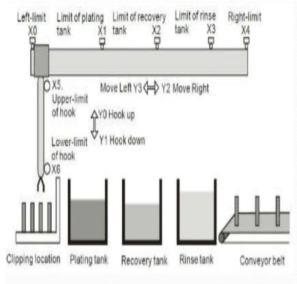
Fig.3: Proposed Block diagram of electroplating
