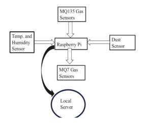
Fig. 7: Overall Design of IoT Prototype
