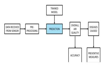
Fig. 1: Block diagram of proposed IoT based Air Quality Prediction System
